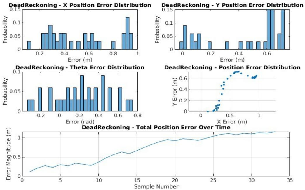
Figure 8. Dead Reckoning - Pose Estimate Error Probability Distributions Compared to Ground Truth
